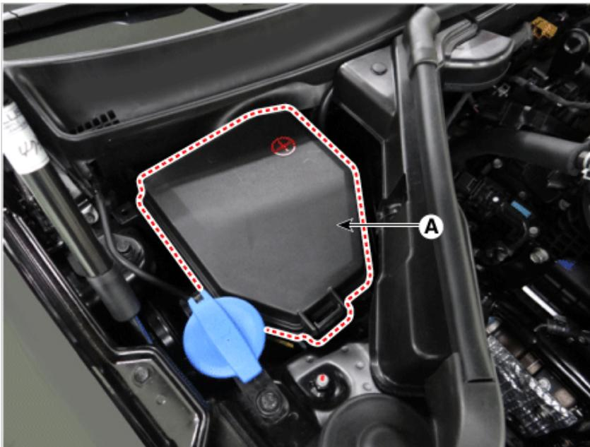
3. Remove the starter relay (A).
