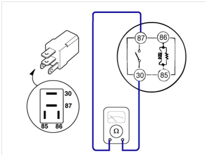
5. Apply 12V to the terminal 85 and ground to the terminal 86 and then check for continuity between the terminals (30 and 87).
